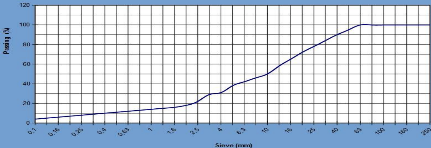
DRAGON 20 Material : Limestone Feeding Size 0 - 1200 mm Rotor Speed : 36 m/sc Adjustment : 40 mm Capacity : 250 - 375 t/h
